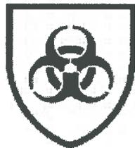
class 6 for the resistance to penetration by contaminated liquids under hydrostatic pressure
